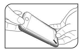
1. Starting from the top right hand corner, install the iPhone into the case.
