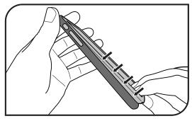
2. Apply the PC bumper onto the TPU body in the same way as shown in the image.
